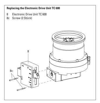
Install the new Electronic Drive Unit TC 600 back onto the turbopump and connect again.
