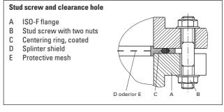
➡ For a flange material having a strength of > 170 N/mm<sup>2</sup> and a stud screw with clearance hole, the nuts must be tightened crosswise in three steps. Tightening torque: DN 100 ISO-F: 5 Nm, 12 Nm, 22 ±2 Nm DN 160 ISO-F: 10 Nm, 20 Nm, 38 ±3 Nm
