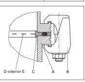
➡ The clamps need to be tightened crosswise in three steps. Tightening torque: 5 Nm, 15 Nm, 25 ±2 Nm
