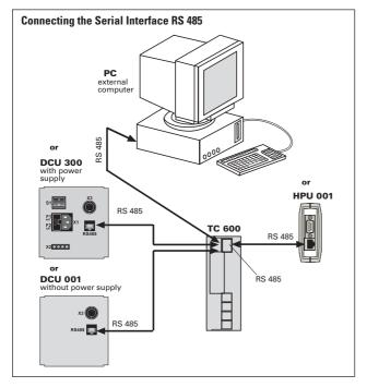
The serial interface is galvanically and safely separated from the maximum supply voltage from the TC 600.
